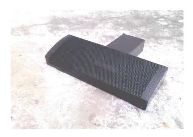
Model PDD diffuser provides a displacement system giving improved air quality and lower temperatures in the occupied zone. The perforated distribution plate provides a constant air distribution over the entire face area without any risk of draught. PDD is designed for installation within the step riser in auditoriums, theatres, cinemas, halls, where good indoor climate conditions are required.
